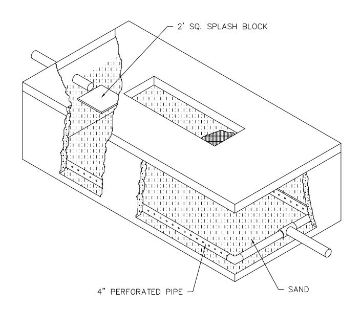
FOR USE AS A POLISHING FILTER. A 82 SQ. FT. SURFACE AREA BY 33" DEEP SURFACE SAND FILTER IS AVAILABLE WITH 24" X 72" GALVANIZED TOP. 76 X 160 X 42" INSIDE, WITH 33" OF FALL THRU THE FILTER.
