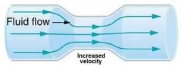
Figure 1. Venturi Effect on a Fluid Through a Constriction
