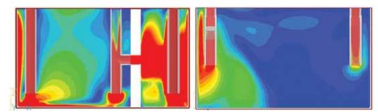
Figure 2. Comparison of Fluid Velocities in Single-Compartment and Two-Compartment Tank When Narrow Transfer Baffle is Used. Fluid velocity is indicated by color (blue is slow, red is fast).
