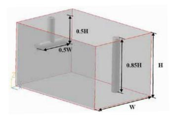
This comprehensive study also shows that local fluid velocities could be reduced by distributing the flow across a larger cross-sectional area. Ideally, the area would occupy the entire cross-section of the of the Figure 3. Example of an Influent Baffle System that Could Distribute the Flow Throughout the Grease Interceptor Tank Figure courtesy of the Water Environment Research Foundation
