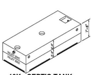
10K - SEPTIC TANK (OUTSIDE DIMENSIONS: 27'-4"L x 11'-6"W x 7'-6"H) [26.75 cu. yd.]
