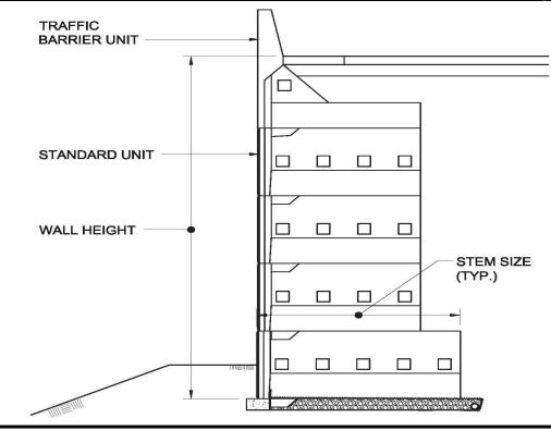
Roadway Surcharge, Backfill Unit Weight  $\gamma$  = 120 PCF
