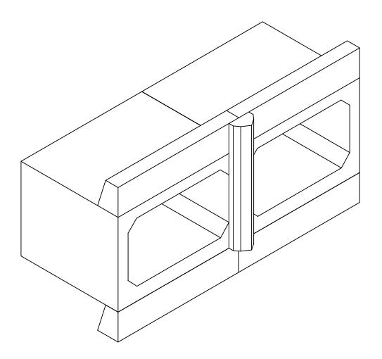
PRECAST FACE — HEAD WALLS AND TOE WALLS CAN BE ASSEMBLED FROM PRECAST CONCRETE COMPONENTS. A PRECAST NOSE SECTION IS AVAILABLE FOR ALL MULTIPLE CELL INSTALLATIONS FOR BOTH INLET AND OUTLET.
