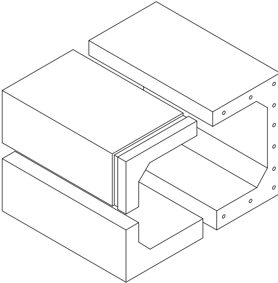
A WIDE VARIETY OF END SECTIONS ARE AVAILABLE WHICH MAY BE USED WITH ANY CULVERT INSTALLATION. SOME SECTIONS ELIMINATE THE NEED FOR ANY CAST IN PLACE CONCRETE.
