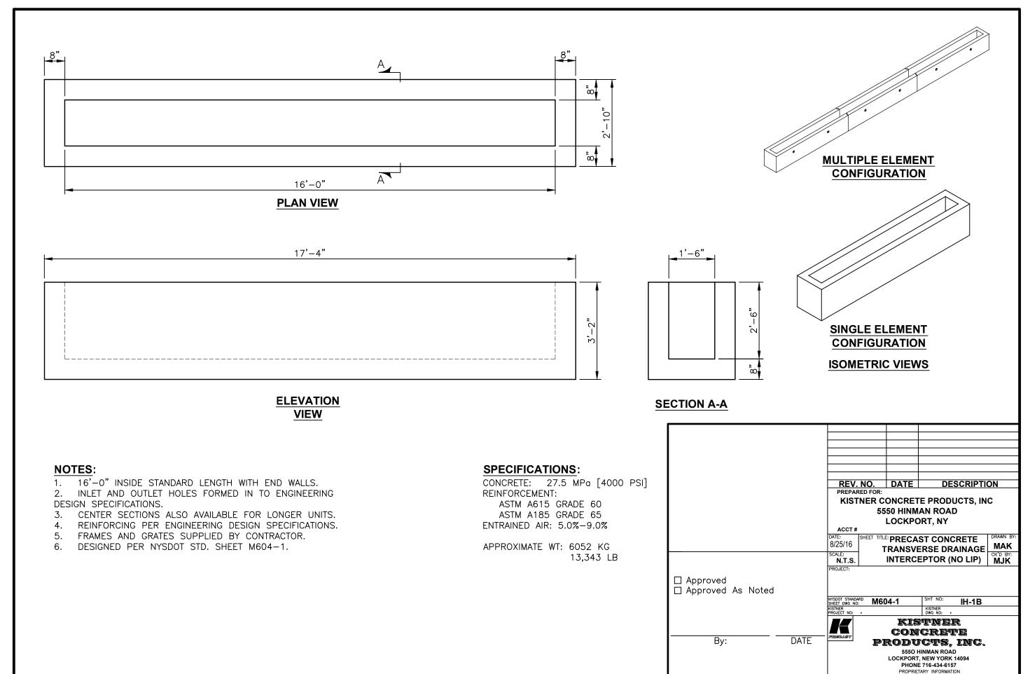
CADD\PRODUCTS\TRENCH DRAIN\18 in TRENCH DRAIN - NO FRAME RO.dwg
