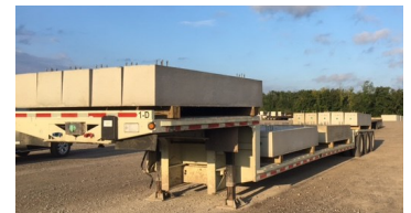
Slabs loaded for delivery.
