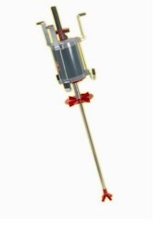
AERATOR 700++ The aerator mechanism is a JET Model 700XX complete with 1/3 HP, 115 volt, 60 cycle, split—phase motor (totally sealed against the entrance of outside water) and stainless steel shaft with a PVC plastic aspirator, corrosion—proof foam restrictor and direct, close—coupled stainless steel drive mechanism as manufactured by JET Inc.
