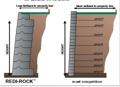
Massive, one-ton Redi-Rock blocks harness the power of gravity to build tall, engineered gravity walls that don't require geogrid in many applications! Redi-Rock gravity walls install like giant Lego walls and can be built close to property lines because they minimize required excavation. Visit <a href="www.redi-rock.com">www.redi-rock.com</a> today for more information on gravity solutions from Redi-Rock.
